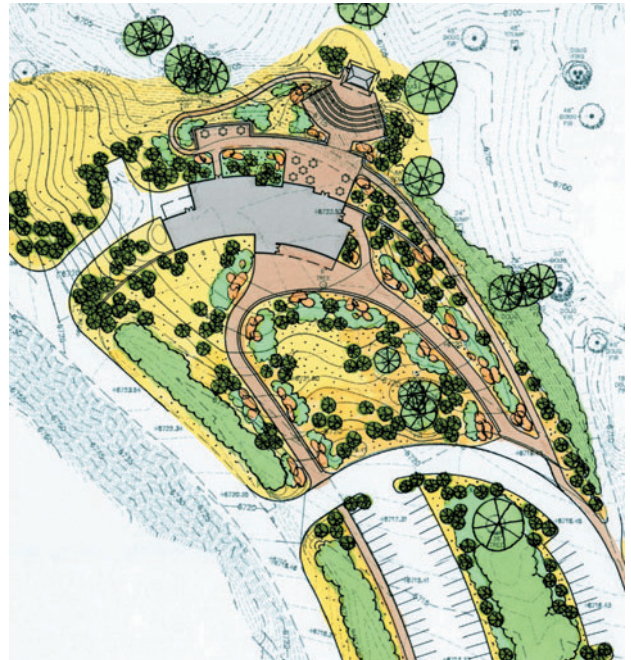
Alternative site plan for curved two-story building scheme minimizes grading while providing ADA-accessible paths and entries, along with an outdoor exhibit landscape of mountain meadow habitats and winter vehicular drop-off at entrance.
